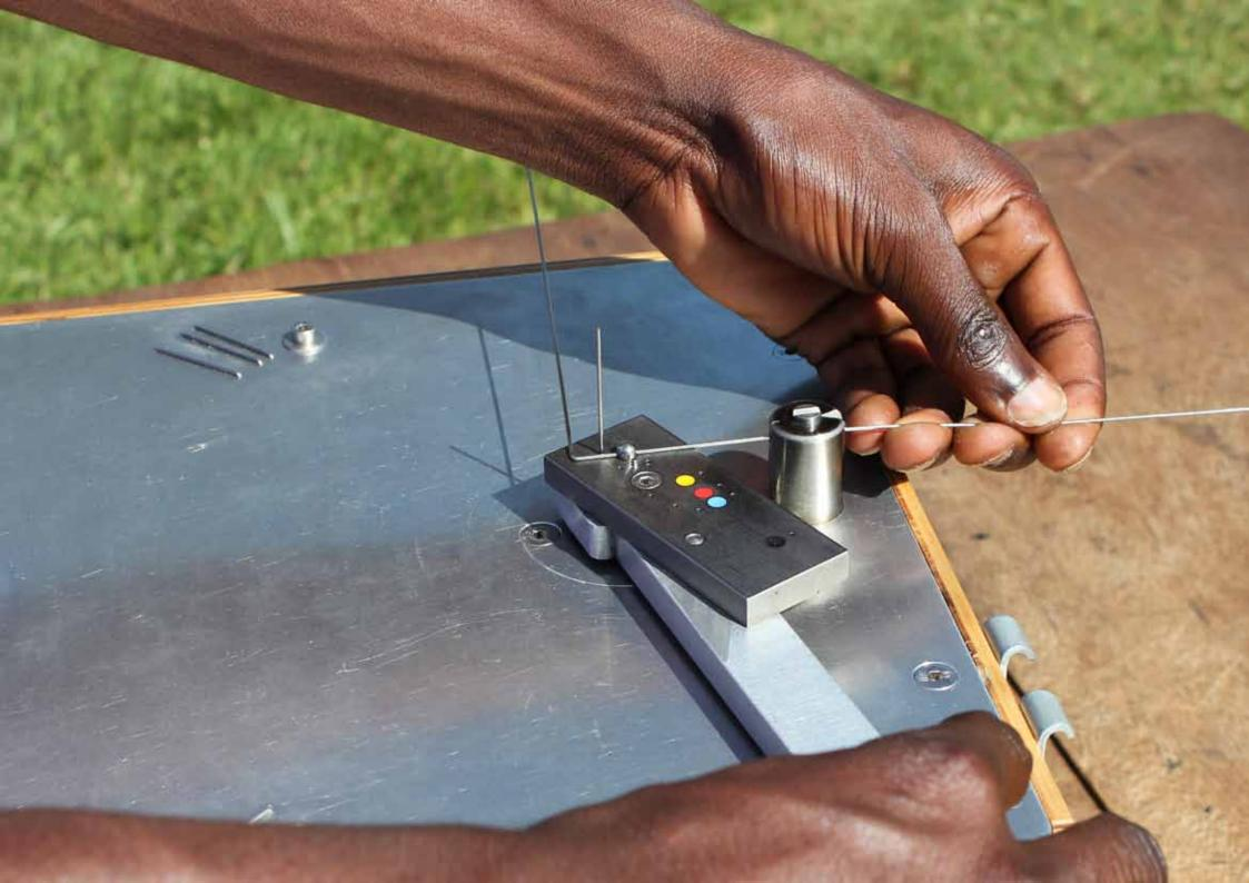
Measuring 4 mm by bringing 4 mm stick into the corner of the wire
